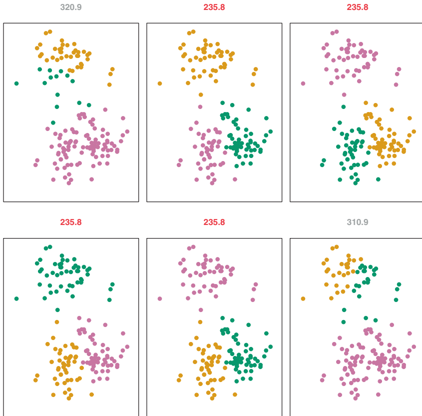
FIGURE 10.7. K -means clustering performed six times on the data from Figure 10.5 with K = 3 , each time with a different random assignment of the observations in Step 1 of the K -means algorithm. Above each plot is the value of the objective (10.11). Three different local optima were obtained, one of which resulted in a smaller value of the objective and provides better separation between the clusters. Those labeled in red all achieved the same best solution, with an objective value of 235.8.
